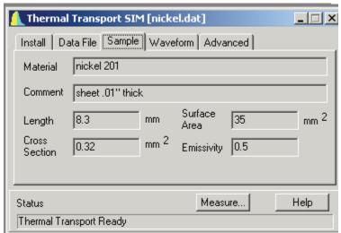
The **Sample** tab displays the sample name, comments, geometry and radiation estimates for the currently open data file. These parameters can be changed only by opening a new file in the **Data File** tab. Chapter 4 has more information on how to mount sample leads and estimate properties such as the sample's infrared emissivity.
