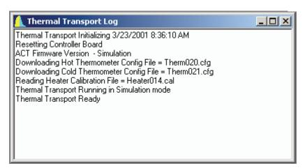
Figure 3-1. Thermal Transport Log Window
