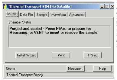
The **Install** tab automatically opens when the software starts, and it assists you in sample installation or removal by providing sample chamber **Vent** and **HiVac** buttons and by also providing an install wizard with more extensive, step-by-step instructions for setting up a measurement.
