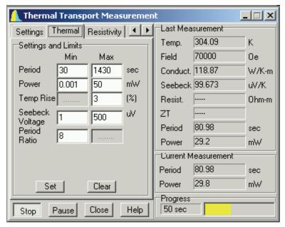
Figure 3-8. Thermal Tab in Thermal Transport Measurement Dialog Box
