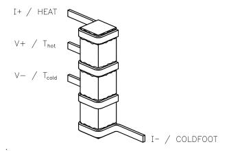
Figure 4-2. Example of Leads Mounted in Four-Probe Configuration
