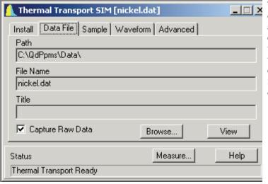
The **Data File** tab lets you open a new TTO data file or append to an existing TTO data file. You can also use the tab to view data and select whether raw thermal transport data is saved in a .raw file. See Section 3.4 for information on TTO data file formats
