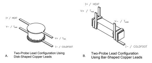
Figure 4-1. Examples of Leads Mounted in Two-Probe Configuration
