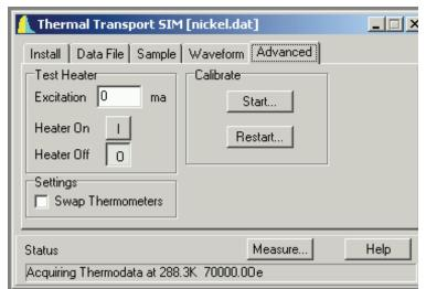
The Advanced tab includes a software wizard that allows you to calibrate new TTO shoe assemblies (heater and/or thermometers) in the PPMS. The calibration fixture (3084-576) from the user's kit is used in conjunction with this software wizard. The Restart... button is used if you previously cancelled a calibration and want to restart. Refer to Section 2.5 for more information on calibrating shoe assemblies.
