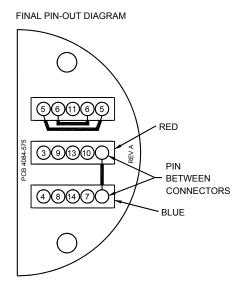
Figure C-2. Top View of Pinout of Connector Sockets on Thermal Transport Sample Puck
