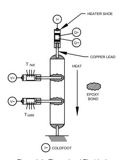
Figure 1-1. Thermal and Electrical Connections for an Idealized Sample
