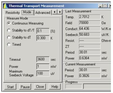
You use the **Mode** tab to select whether to take continuous measurements (default) or single, steady-state measurements. There are two modes of single measurement: stability or timed. Section 1.3 describes the measurement modes in more detail.
